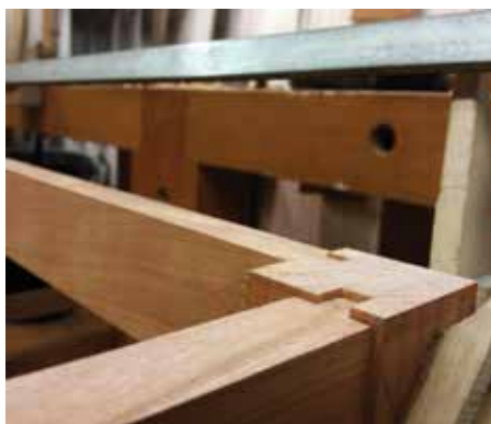
Mitred and haunched mortise and tenons provide a very strong joint between the legs and the aprons
