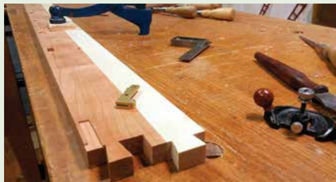
Installing knife hinges on the upper apron before adding the edge inlay
