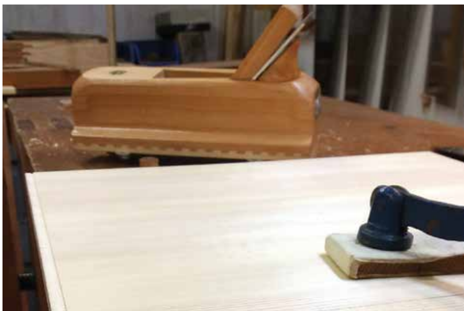
A wooden dovetail plane is used to create the male part of the sliding dovetail
