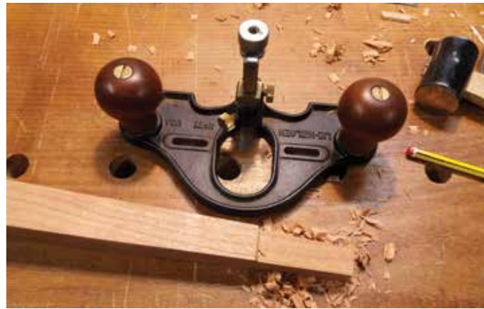
Using the router plane to make space for the cocobolo sabot feet
