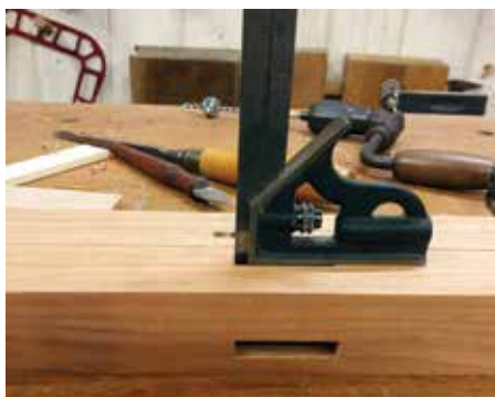
Checking the mortises with the combination square
