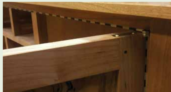
Knife hinge mounted on door and apron
