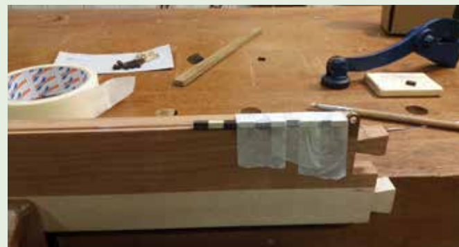
Gluing ebony and holly dots with the knife hinge fixed
