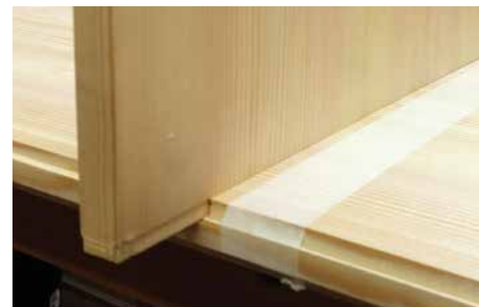
Keep the male panel over width until a good fit has been established. Apply masking tape either side of the dado to prevent the router plane from marking the surface
