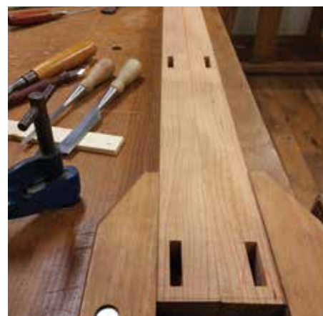
Wooden screw clamps are ideal for supporting the workpiece and help to prevent splitting
