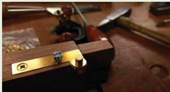
Knife hinge in the lower front apron. Pre-drilling with a steel screw
