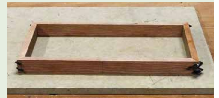
Splines are cut into the corners of the tray after the initial assembly
