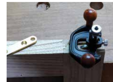
Use a small router plane to let the hinge into the ends
