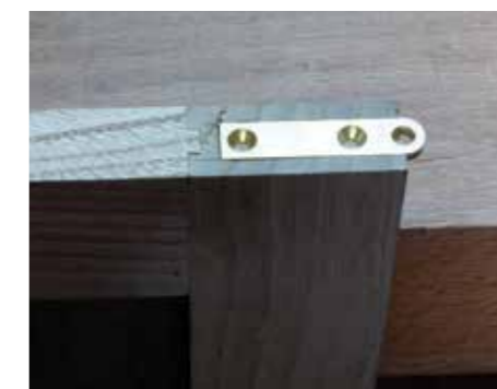
Set the hinge parts flush with the surface of the door
