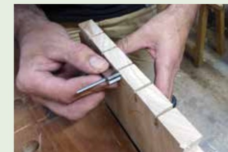
Checking the dovetails
