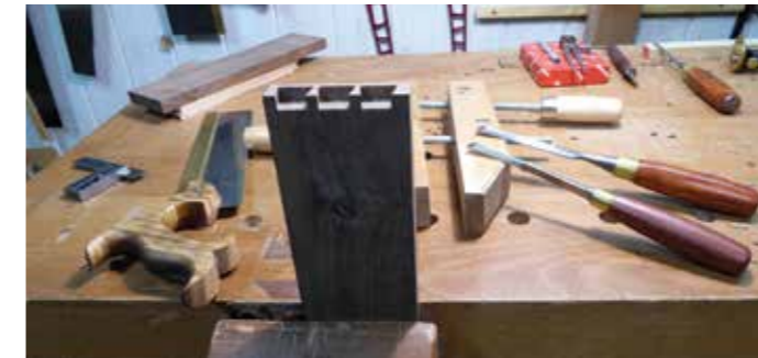
Making the pins on the drawer fronts
