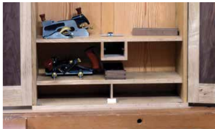
Tools that are used most often are stored on the lower shelves RIGHT: Rare earth magnets keep the planes in place
