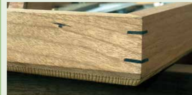
Splines add strength as well as a little detail
