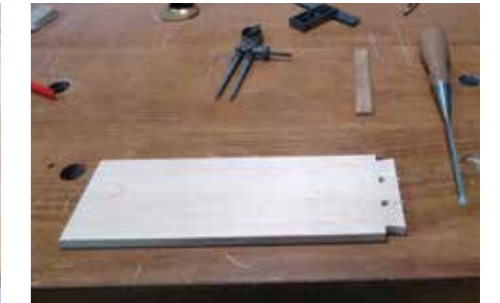
Making the tails on the drawer sides
