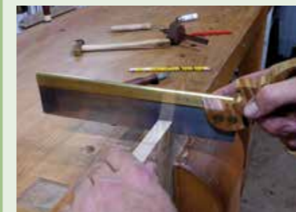
Sawing the dovetails
