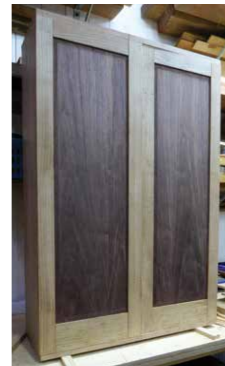
Checking the doors for size before fitting the hinges
